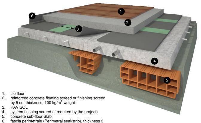
PAVISOL is recommended whenever higher acoustic comfort and impact noise resistance are required.
